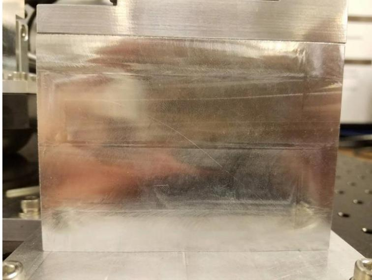
Figure 15. Surface ripples on the gantry support block
