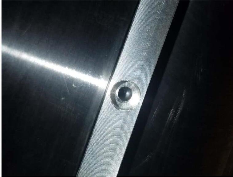
Figure 14. A misaligned hole at the linear encoder code rail mounting block
