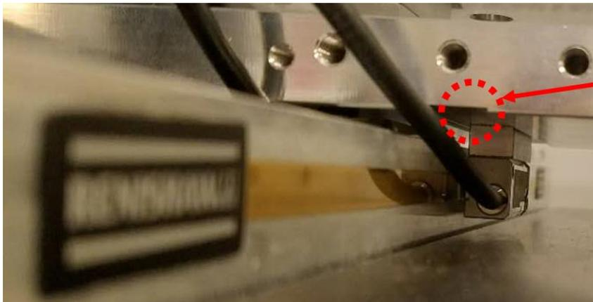
Encoder mounting block and FS touching at the machined plane
