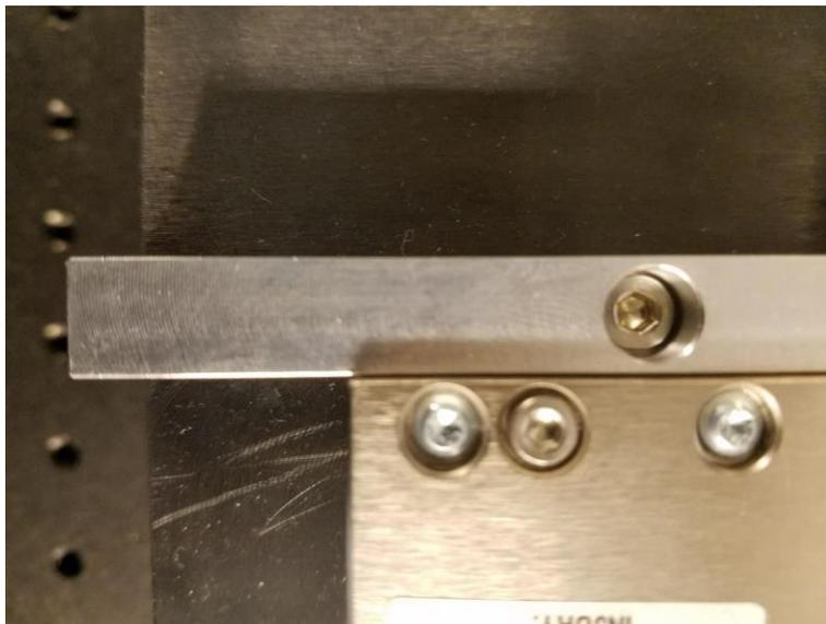
Figure 16. Surface ripples on the linear motor mounting block
