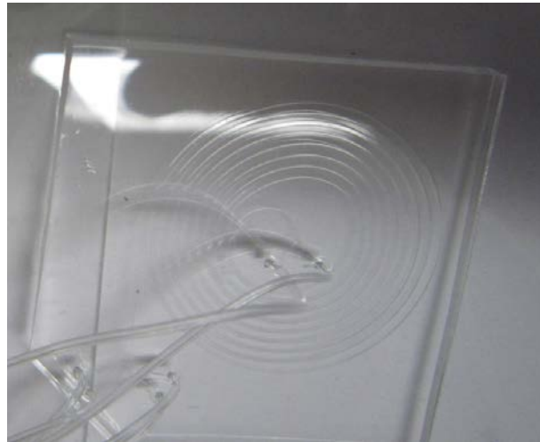
Fig. 2 Microfluidic device with four different outlets. Solutions with cells and particles are run through the device and separate due to differing flow dynamics.
