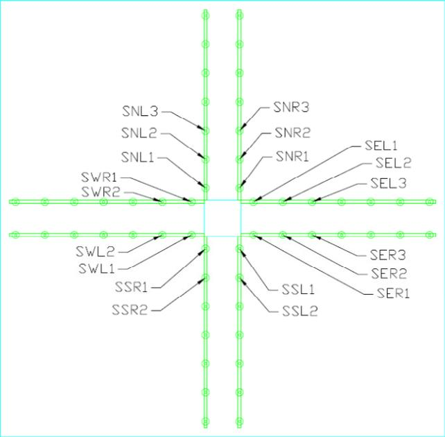
Fig. 3-7 Gauged Studs Locations
