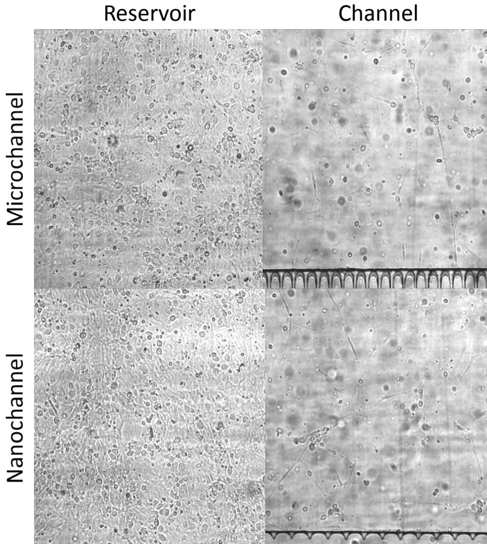
Figure 14: Microchannel and nanochannel devices show comparable growth in reservoirs and channels on day 2
