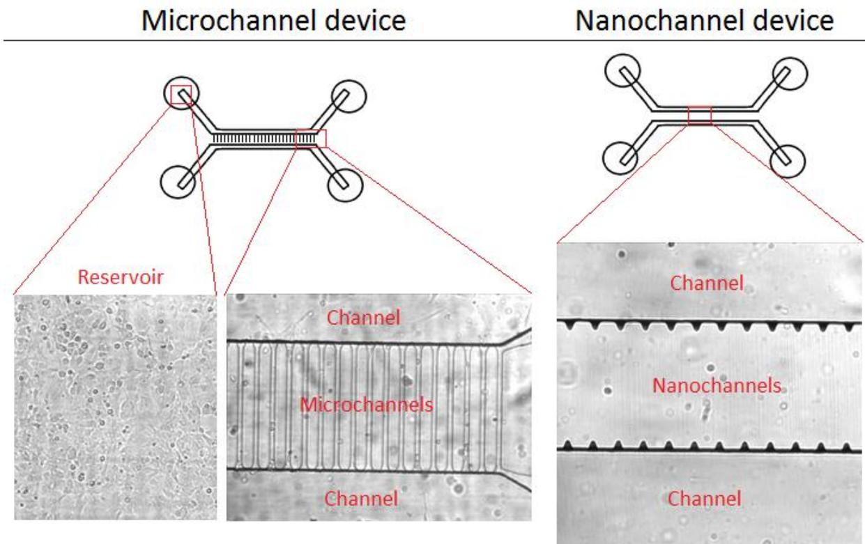
Figure 2: Microchannel device and nanochannel device
