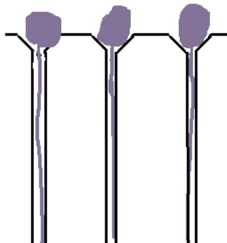
Figure 13: Design to allow spatial separation of cell bodies and axons
