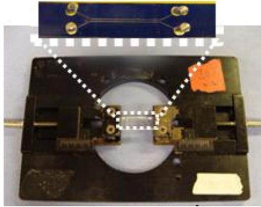
Figure 3: Home-made stretcher loaded with a microfluidic device
