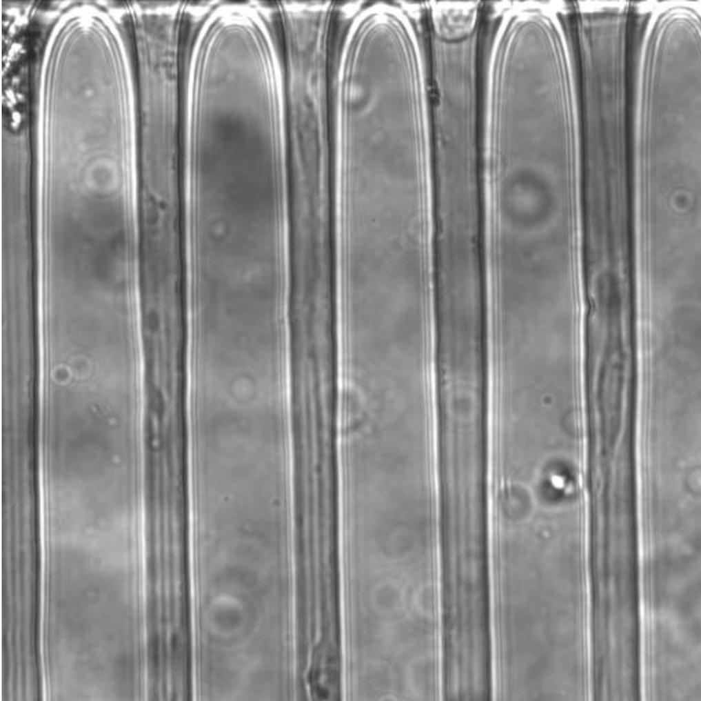
Figure 11: Primary neuron cells growing linearly in microchannels, at 3 days after seeding
