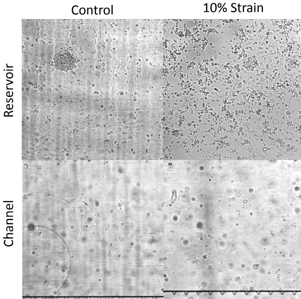
Figure 15: Similar reservoirs growth for control and stretched devices. Only control channels has growth
