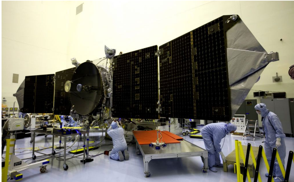
Figure 1. Inside the Payload Hazardous Servicing Facility at NASA's Kennedy Space Center in Florida, engineers and technicians test deploy the twin solar arrays on the MAVEN spacecraft.
