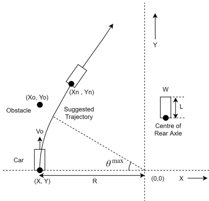
Figure 5: Collision Avoidance System
