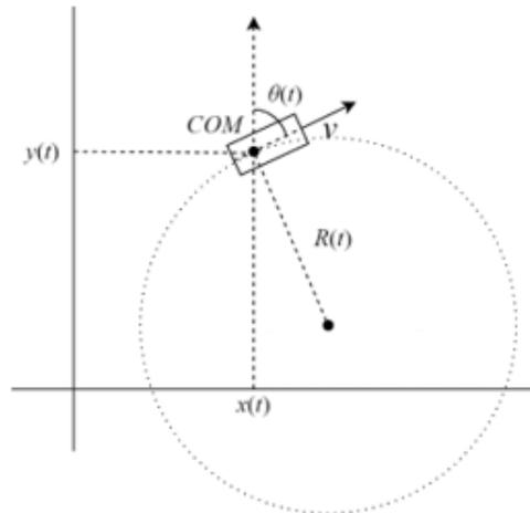
Figure 1: Kinematic Model
