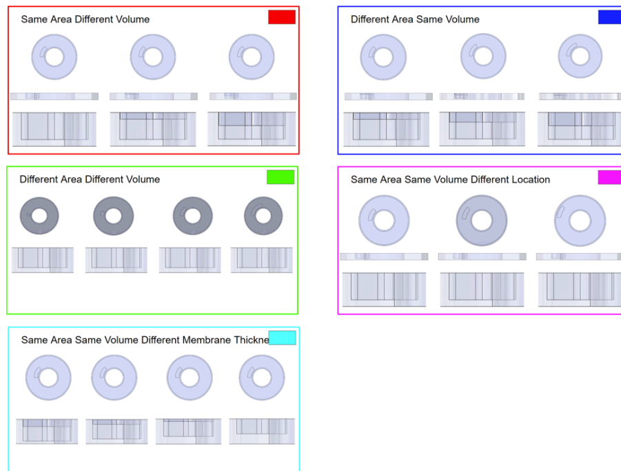
Fig 3. Experiments Design for Detaching Performance of Suction Cup with Different Designs of Secondary Chamber
